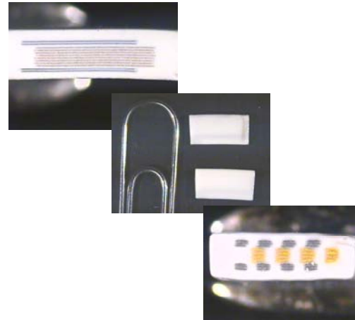
Figure 2: Optical images of band and dash geometries incorporating both gold and platinum materials
