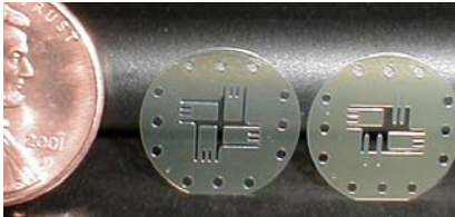
Figure 3: Blank micromachined substrates for sensor arrays.
