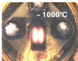
Single packaged sensor in operation in air and its equivalent circuit.
